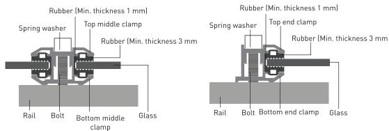
Fig 2: Mounting with clamps
